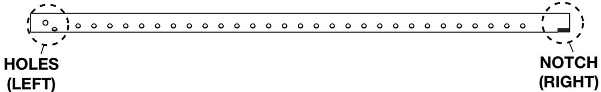
1. With the appliance door open or removed, insert the left side of the secondary air tube into the hole in the **left side** of the appliance.
